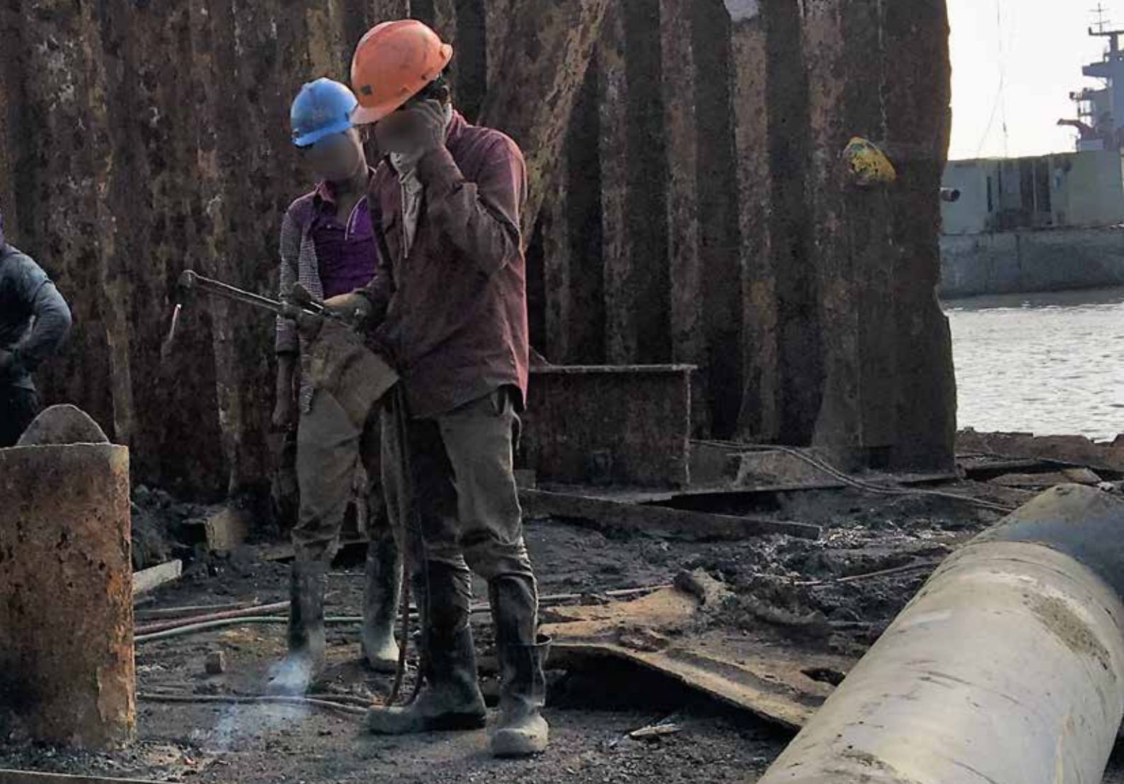
Shipyard workers torch cut at a shipyard in Chittagong. The flame can reach up to 1500 degrees celsius and process can release toxic gases and fumes.
